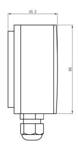
M16 cable fixing connector
