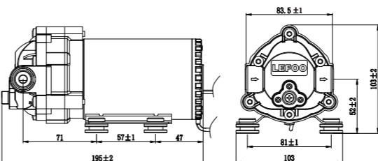
LFP6050-LFP6075W (3/8" NPT)
