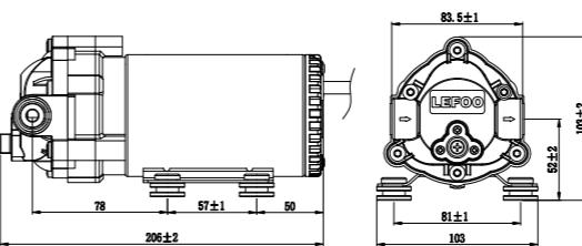
LFP5200-LFP5300W (3/8" NPT)
